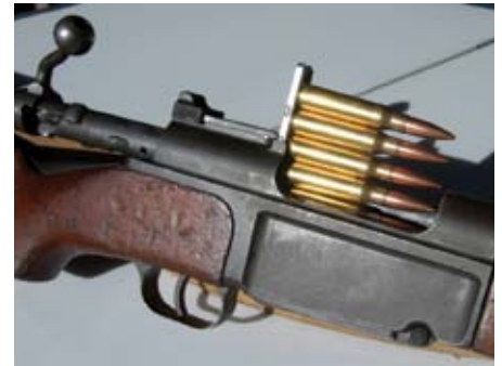
Loading using the charger clip inserted into the charger rail at the rear of the receiver port.
