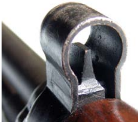
The fore-sight with the tubular protector on an MAS-36 Type 2.
