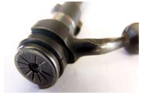
The bolt plug. Note the notch on the bolt collar, the 'D' marking for disassembling and 'M' for reassembling on the bolt plug.
