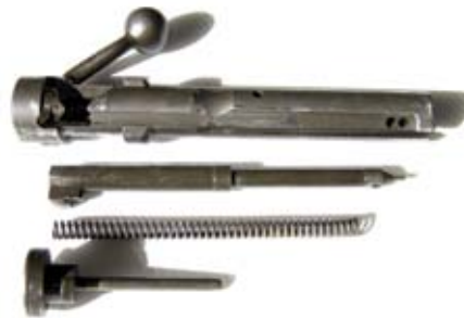
The bolt disassembled, with the bolt body with the bolt handle, the hollow firing pin, the coil spring and the bolt plug. Note the rear bolt lugs and the three gas vents.
