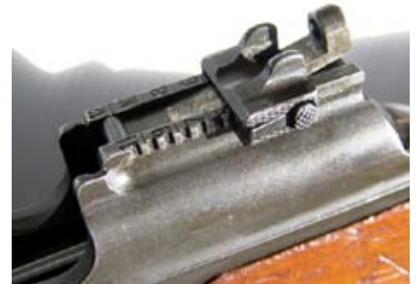
The aperture rear-sight located on the top of the receiver bridge is graduated from 200 to 1200m in 100m increments.
