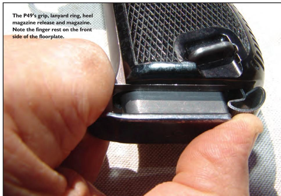
**The P49's grip, lanyard ring, heel magazine release and magazine. Note the finger rest on the front side of the floorplate.**
