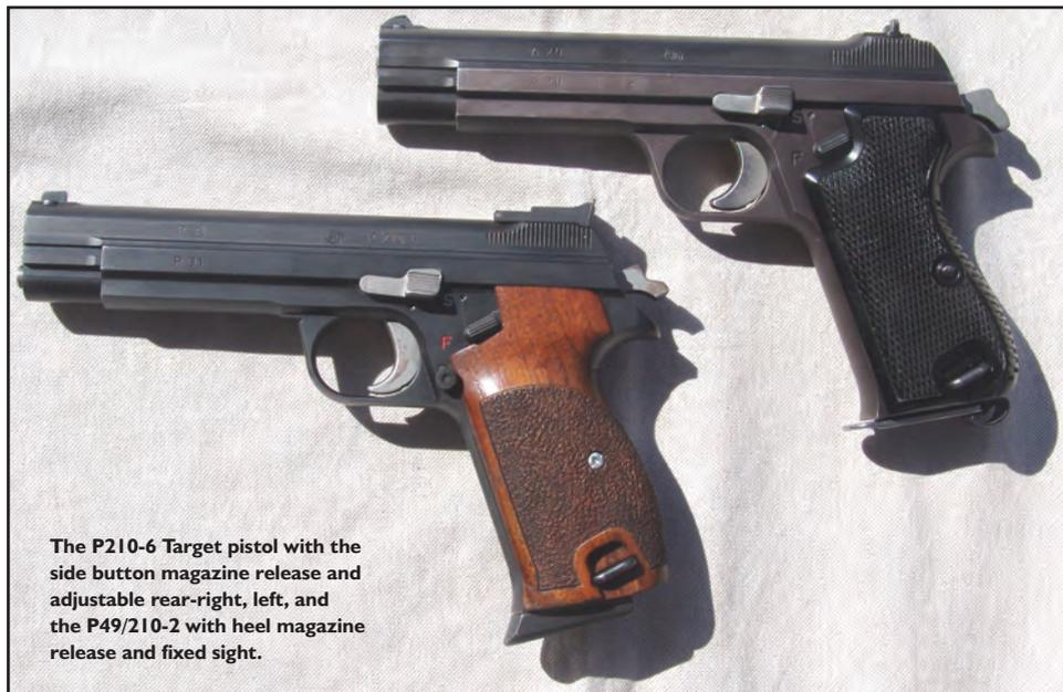
The P210-6 Target pistol with the side button magazine release and adjustable rear-sight, left, and the P49/210-2 with heel magazine release and fixed sight.
