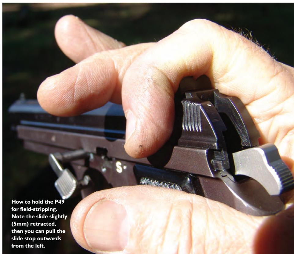
**How to hold the P49 for field-stripping. Note the slide slightly (5mm) retracted, then you can pull the slide stop outwards from the left.**
