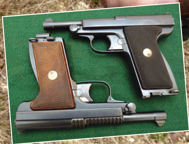
The Le Français original Army self-loading double-action pistol, top, and the 1931 model with the grooved barrel.
