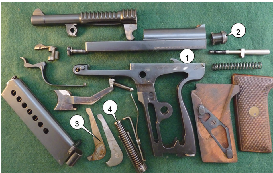
The Le Français 1931 Army model field-stripped: 1. The extractor fixed on the frame, 2. The rear and slide plug maintaining the firing pin and its spring in the slide, 3. The recoil rocking levers, 4. The recoil spring.
