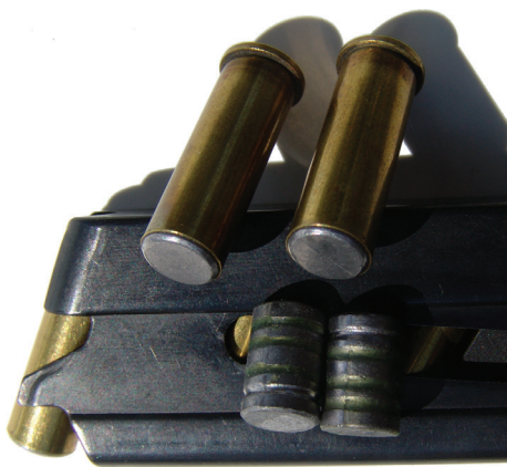
The five-cartridge P240 magazine shown with home-casted RCBS .38 SPL WC (ref 82030) bevel base and nose, resized .357 and lubed.
