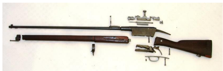
Photo 3: The Lebel 1886 M 93 taken to parts with the bolt, the receiver (containing the repeating and trigger mechanism) linking the two stock parts
