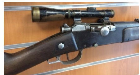
Photo 11: Sniper Lebel rifles with a 3x magnification APX Mle 1915 or 1916 scope
