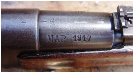
Photo 9: Photo 10: The barrels manufacture and date (with the post-1932 N stamp)
