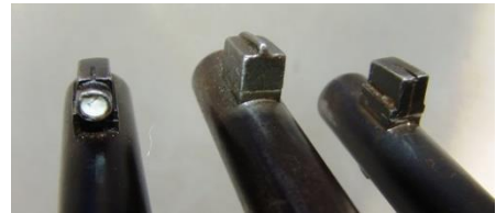
Photo 7: Different Lebel front sights (grooved/luminescent (1917), post, and grooved)
